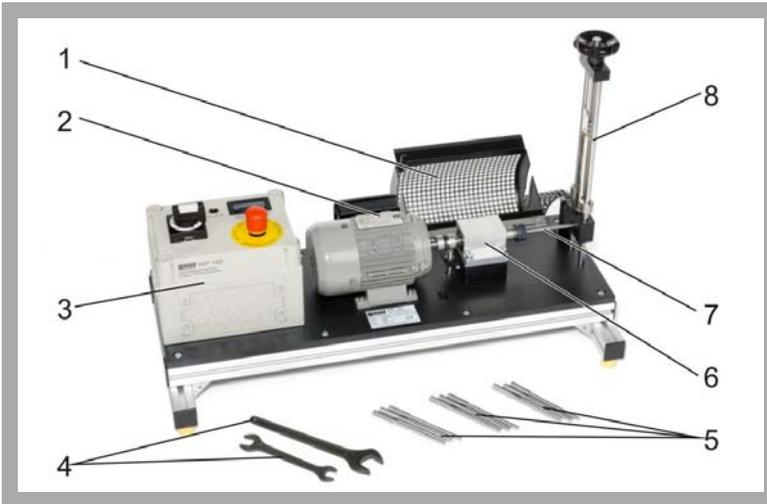
1 protective hood, 2 drive motor, 3 switch box, 4 tools, 5 test bar, 6 support, 7 test bar, 8 loading device with spring balance and hand wheel for adjustment
