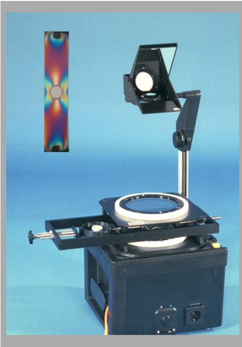
The picture shows the FL 210 unit with a standard commercially available overhead projector (not supplied).
