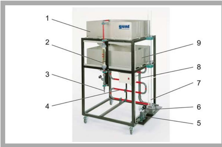
1 basin A with adjustable weir, 2 flow meter, 3 water connection, 4 drainage line, 5 gate, 6 valve, 7 surge chamber, 8 overflow pipe, 9 basin B with overflow
