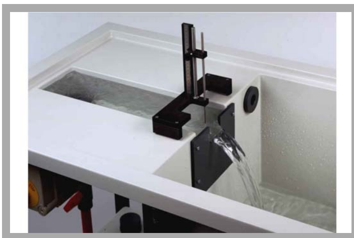
Base module for experiments in fluid mechanics with HM 150.03 plate weir
