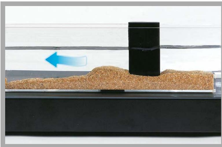
Fluvial obstacle mark (scour formation and siltation) on piers
