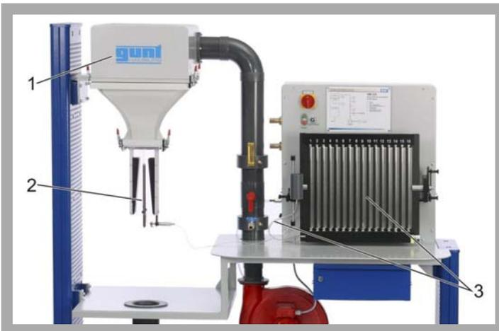
Experiment setup: 1 HM 225, 2 HM 225.02, 3 tube manometer (HM 225.01) with connection to HM 225.02
