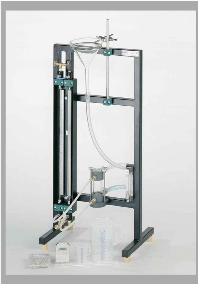
**\* Cake and depth filtration with different suspensions and filter medium layers**
